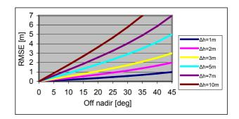
Figure 4. Presents quantitative influence of de-leveling in function of the optical system deflection angle
