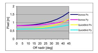
Figure 2. Terrain size of pixel in function of the camera deflection angle for the systems IKONOS and QuickBird
