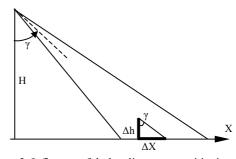
Figure 3. Influence of de-leveling upon positioning on the image.
