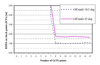
Figure 7. Accuracy of IKONOS for parametric approach
