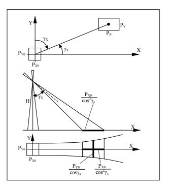
Figure 1. Influence of the angle of optical system deflection upon the land size of pixel of image and on the width of the imaged strip.
